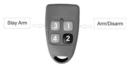
The functions that can be assigned to a button are: arm/disarm, stay, relay 1, and relay 2. Each button can be assigned multiple functions, or no function. It cannot be assigned both arm/disarm and stay. Different buttons can be assigned the same function.
