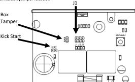
**NOTE**: If J1 is shorted after the system is powered on, please repower the system with J1 shorted to enable serial communication
