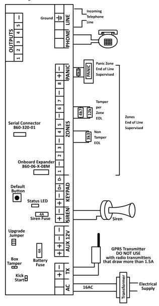
**Note:** When using extra power supplies to power any peripheral connected to the keypad bus an IDS RS485 isolator (860-06-0557) must be used.
