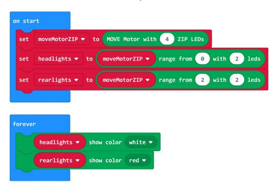
**STEP 4:** If you have a micro:bit connected, click "Download" to transfer your code. Then switch on :MOVE Motor and see the lights turn on!
