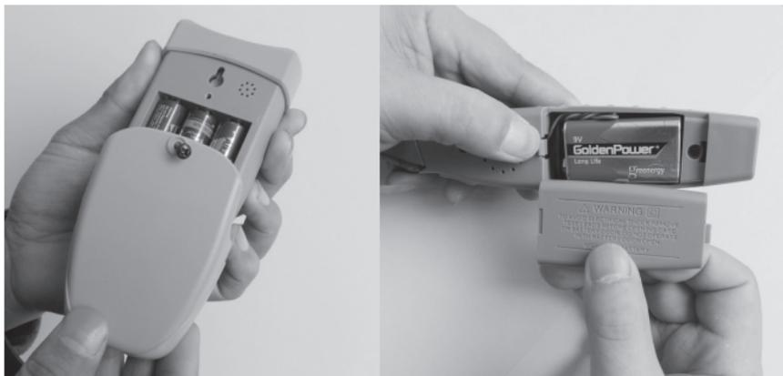
Replace the 3 x 1.5V AA (R6) batteries for the transmitter and 1 x 9V (6F22) battery for the receiver.
