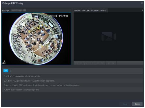
Step 5 Click and then move the of the fisheye on the left to select a position. Click of the PTZ camera to find the position. Adjust the PTZ camera to find the position and move the PTZ to the center position (The green cross on the image).
