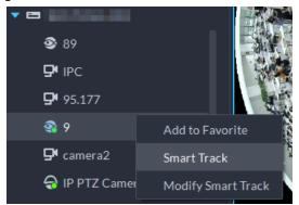
Step 2 Click any point on the left of fisheye, PTZ camera on the right will automatically rotate to corresponding position.
