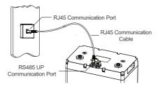
If the monitoring screen is used with a parallel battery bank, the communication between paralleled batteries must be enabled. Please connect the RS485 LINK Communication Ports of the former batteries to the RS485 UP Communication Ports of the latter ones using CAT5 (or above) Ethernet straight through cables (not included). The monitoring screen should be connected to the RS485 UP Communication Port of the first battery.
