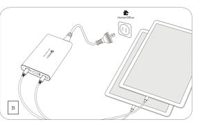
Caution: This adapter supports power 60W max.lf your used power exceeds 60W the adapter will occur to be over-load protection. When you re-plug the connection,
