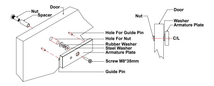
Important: Do not fix the armature plate too tightly. Make the rubber washer flexible, in order to ensure the armature plate automatically adjusts to its proper position with the magnet.
