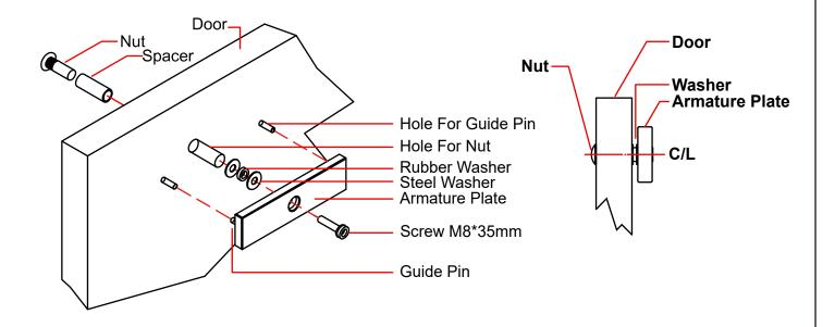
Important: Do not fix the armature plate too tightly. Make the rubber washer flexible, in order to ensure the armature plate automatically adjusts to its proper position with the magnet.
