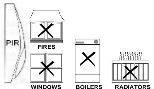
Do not site a PIR where its field of view may be obstructed (e.g. by curtains). Also note that PIRs work best when sensing movement across rather than along their detection beams. You need to consider the need to wire these units back to the Control Unit.
