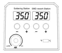
1. Press the button "+" or "- " to adjust the temperature.
