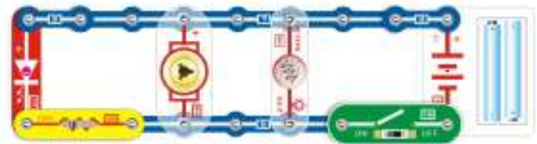
29. Parallel connection of lamp, LED and motor
