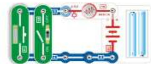
55. Two switches in parallel control one lamp
