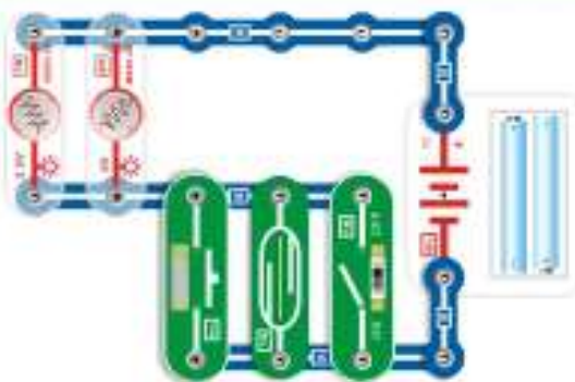
69. Three switches in parallel control two parallel-connected lamps Turn on any one switch can light the two parallel-connected lamps at the same time; the bulb can be go out only when all three switches are turn off.
