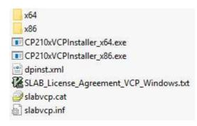
Select the "CP210xVCPInstaller\_x64.exe" and go through the setup prompts to install the driver.
