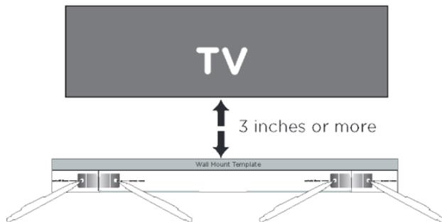
2. Remove the template, using an appropriately sized drill bit, drill a hole in the wall at each marking.
