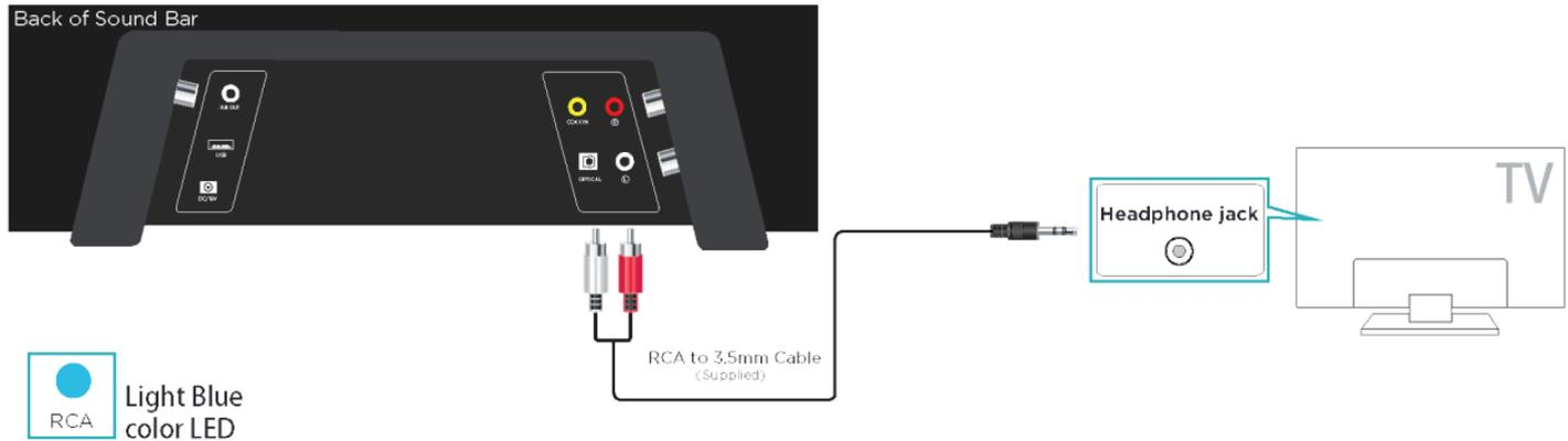
1. Connect RCA(L/R) on the Soundbar to the AUDIO OUT(3.5mm Headphone) jack of the Source Device using a RCA to 3.5mm cable.
