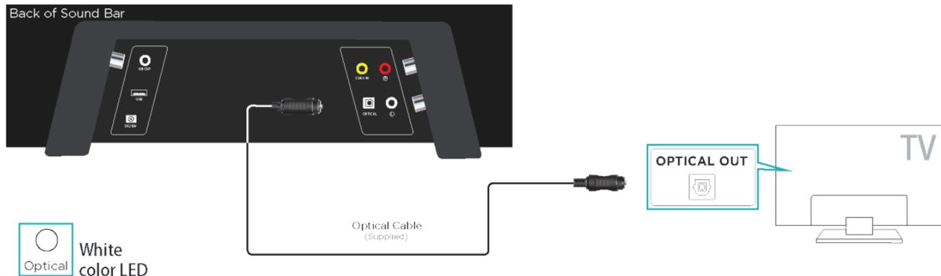
1. Connect the DIGITAL AUDIO IN(OPTICAL) jack on the Soundbar to the OPTICAL OUT jack of the TV with a digital optical cable.
