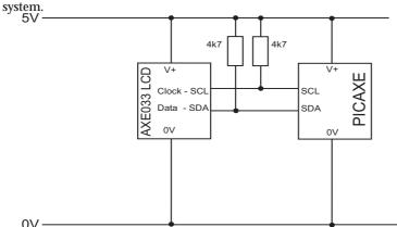
Note that the 4k7 resistors pull up resistors are pre-soldered onto the AXE033 LCD module. Therefore additional external resistors are not required.
