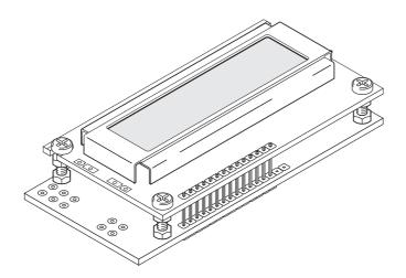
The serial LCD and clock module allows microcontroller systems (e.g. PICAXE) to visually output user instructions or readings, without the need for a computer. This is especially useful when working, for example, with analogue sensors, as the analogue reading can easily be displayed on the LCD module. All LCD commands are transmitted serially via a single microcontroller pin using the **serout** command. e.g.
