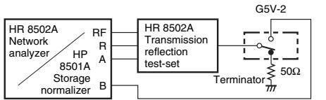
Terminals which were not being measured were terminated with 50 Ω.
