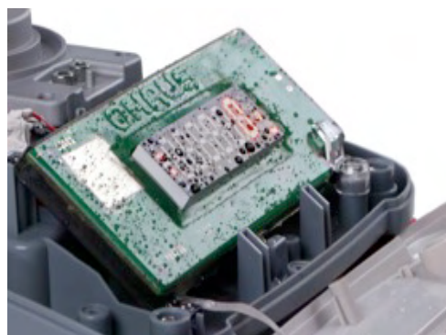
Inside PCBA Silicon Glue Sealing
