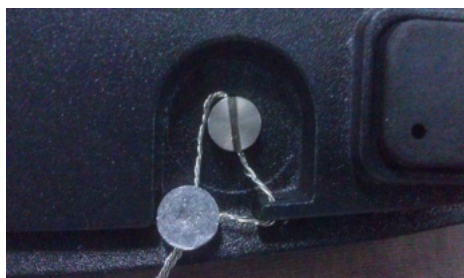
Locked with Wire Seal
