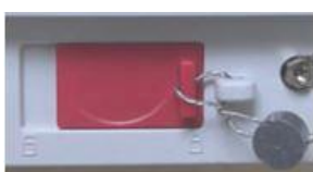
Locked with Wire Seal
