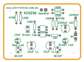
Using the component overlay, the component list and the circuit diagram load and solder the components into the printed circuit board (PCB).
