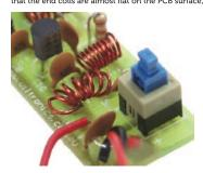
When you have peaked L3 for maximum output remove the circuit and solder the antenna lead in its place. If you change transmitting frequency then you will need to repeat the peaking procedure in order to get maximum power output.
