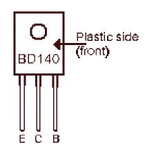
The BD140 transistor supplied may not have E, C, B marked. Please see diagram for pinout.
