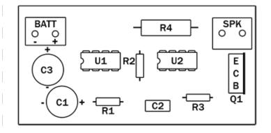
Using the component overlay, the component list and the circuit diagram load and solder the components into the printed circuit board (PCB).
