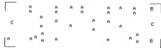
Fig 3. Hole Size Map shows a total of 34 holes. (View from copper side) 2 x size A = 1.00mm, 2 x size B = 5.0mm and 30 x size C = 0.8mm. (not to scale)
