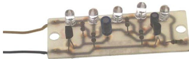
Fig 5. Component overlay shows the component positions and polarities with a view of the copper tracks from the component side of the PCB.
