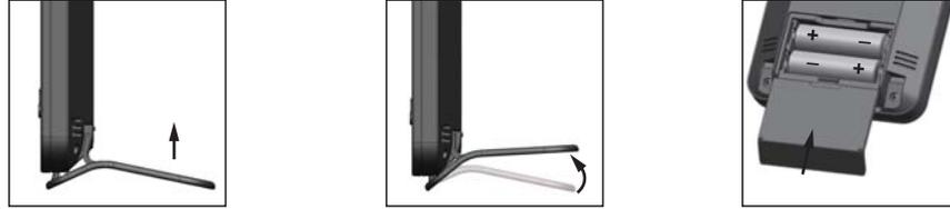
1. Remove the battery door of the main unit.
