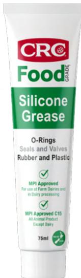
**CRC Food Grade Silicone Grease** is a thin non-curing silicone grease designed for sealing, lubricating and waterproofing o-rings and other rubber and plastic parts used in food processing equipment.
