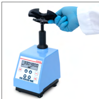
2. Put tube holder onto shaft
