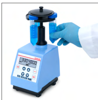
5. Check if tubes are firmly clamped
