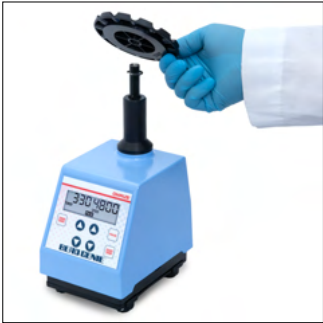
2. Put tube holder onto shaft
