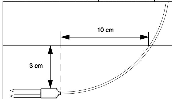
Do not bend the cable too severely when putting the probe into the soil. Let about 10 cm of the cable nearest to the probe remain straight or gently curved as shown.
