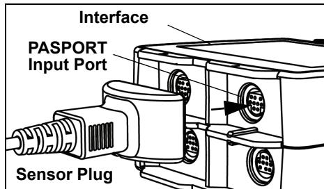
NOTE: If more distance is needed between the sensor and the interface, plug the sensor into a Sensor Extension Cable (PS-2500) and then plug the cable into the interface.
