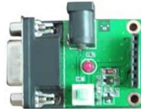
When configuring module, users should insert the module into RS232 converter board correctly and connect it to PC and then open software tool. After the tool finds the module and shows “Found device” in the status line at the bottom, users then can write/read modules through corresponding buttons. After successful operation, the message “Write succeed” or “Read succeed” will be showed in the status line.
