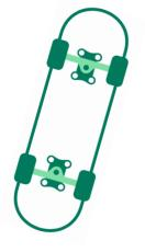
The whole underside of the board would be in contact with the ground, creating a lot of friction. When you add the wheels to the skateboard, only the wheels touch the ground. There is a lot less friction, meaning it takes less effort to move.
