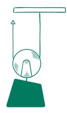
Because the load is attached to the pulley, the pulley moves with the load. This means that the pulley and the load are supported by two sections of the same rope. This multiplies the force, reducing the effort required to move an object vertically.
