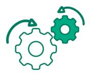
Gears can also be connected in different ways (such as perpendicularly to each other) to change the direction of a force, sending it off in a different direction. There are also special gears that are used to send the force from a power source off at an angle.
